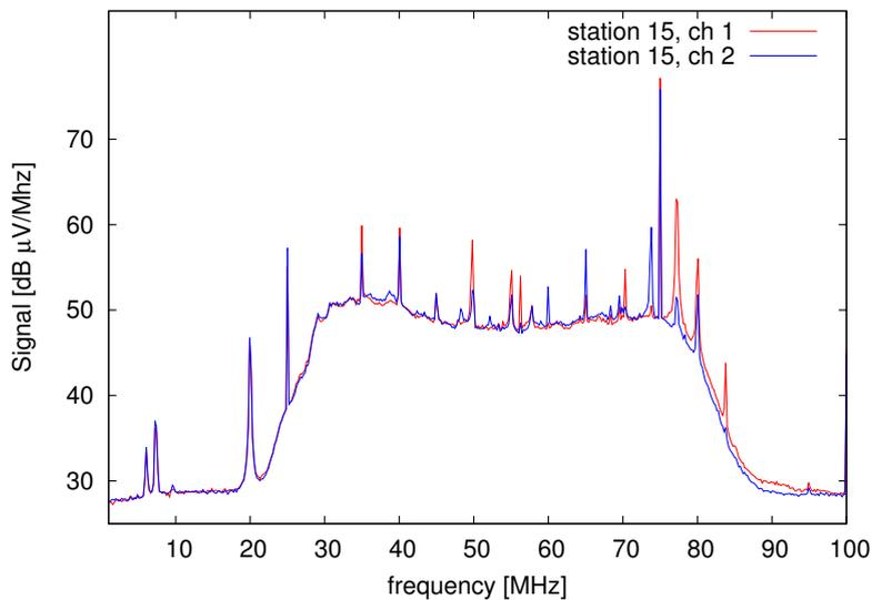
Fig. 3. Mean background spectrum of a Tunka-Rex station over on typical night. A filter attenuates the signal outside the design band of 30-80 MHz. Several narrow band noise sources lie within this band, of which currently only some are identified. However, they can easily be suppressed digitally during data analysis.
