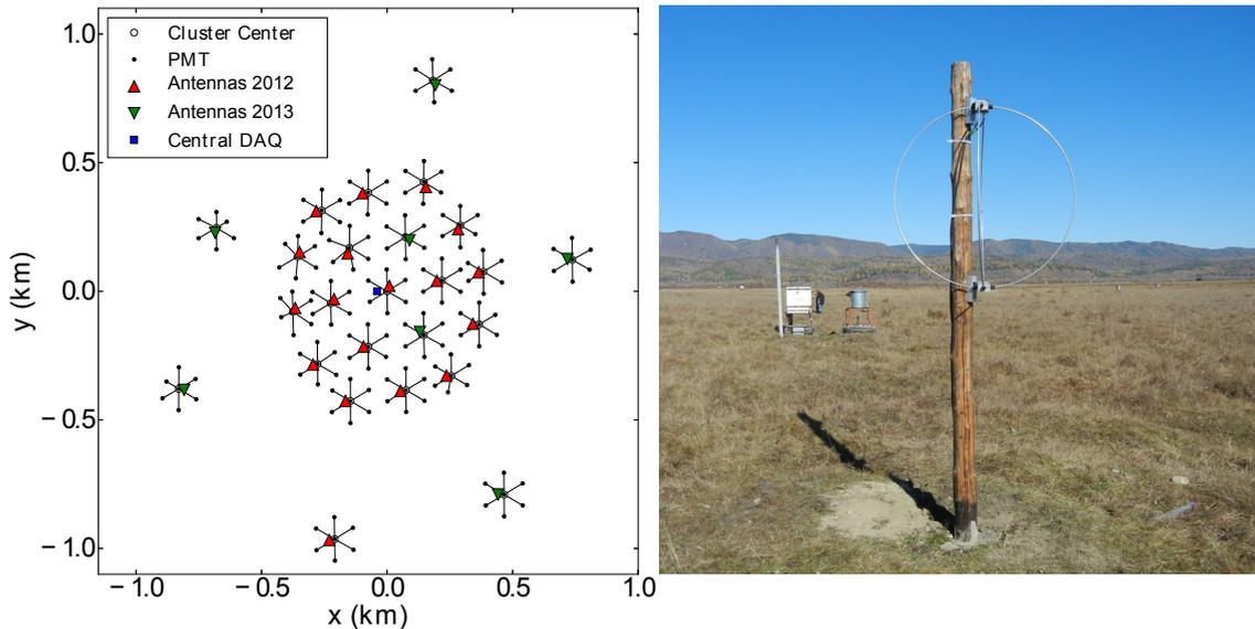
Fig. 1. **Left:** Map of the Tunka-133 and Tunka-Rex detector layout with installation date of the antennas. **Right:** A Tunka-Rex antenna station in front of the central PMT and the DAQ of one of the 25 Tunka-133 clusters, and the cluster center.
